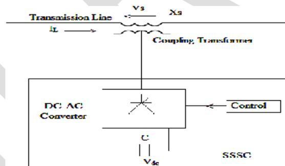
Fig.3. Static synchronous series capacitor
