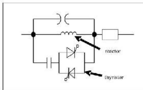
**Fig.2. Thyristor-Controlled Series Capacitor**
