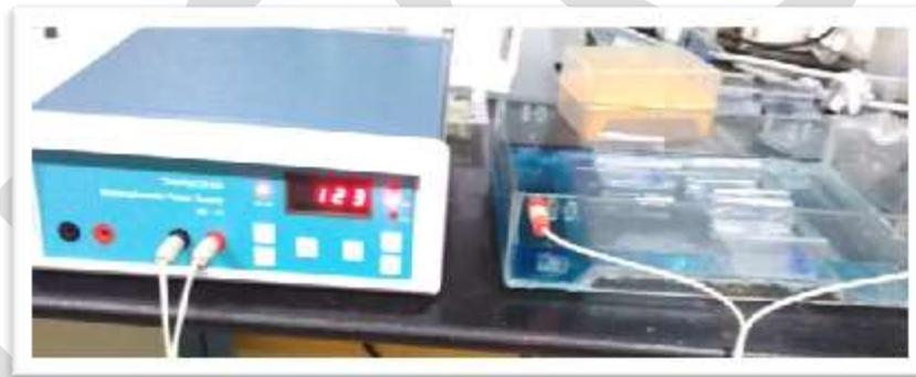
*Fig. 12. Gel electrophoresis unit*
