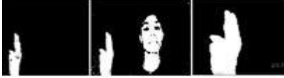
Fig 3 a) Foreground image a) Difference image b) Color space segmented image c) Hand gesture image
