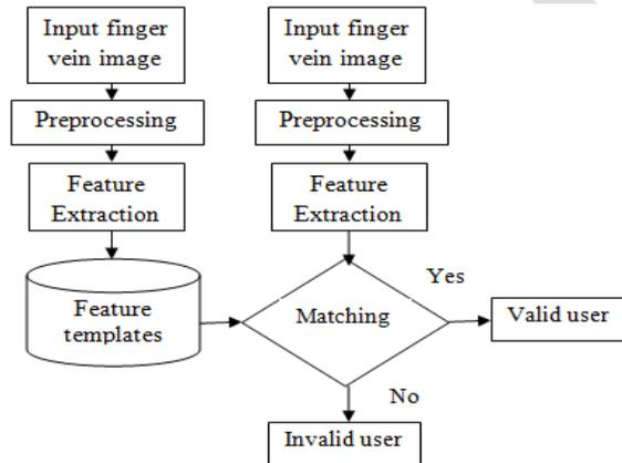
**Figure 2 Flowchart of finger-vein authentication system**
