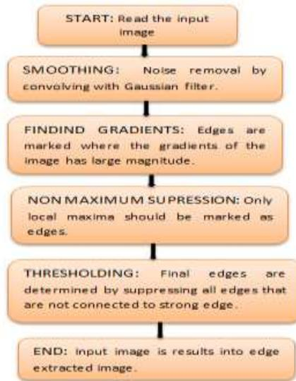
*Figure 4 canny edge detection algorithm*
