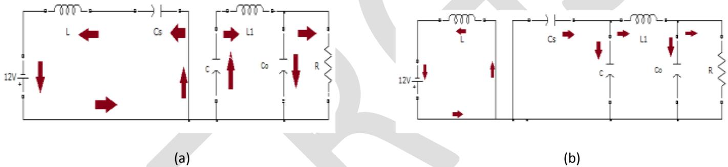
Equivalent circuits. (a) Switching ON. (b) Switching OFF.
