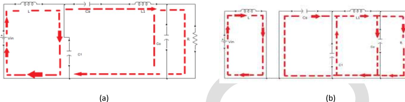
Equivalent circuits. (a) Switching OFF. (b) Switching ON.
