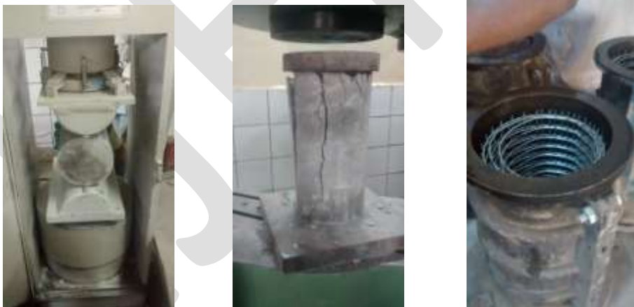
Fig 4.1 & 4.2 Specimen at Testing & mesh in cylinder mould.
