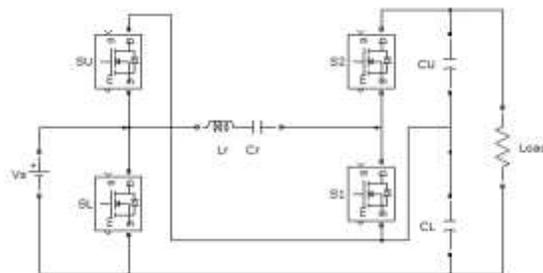
Fig.2 Bidirectional DC-DC converter using resonant PWM
