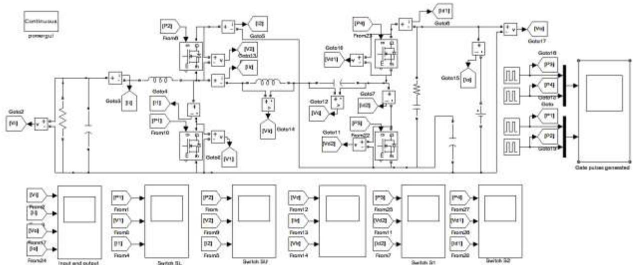
Fig.9 MATLAB/Simulink model of bidirectional converter in buck mode
