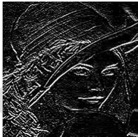
Figure 3. Output of Prewitt operator
