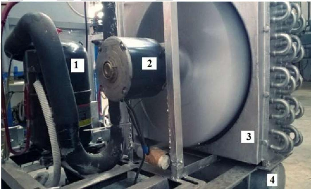
**Figure 1** Various Components of Cold Storage: 1. Compressor, 2. Fan, 3. Condenser and 4. Receiver
