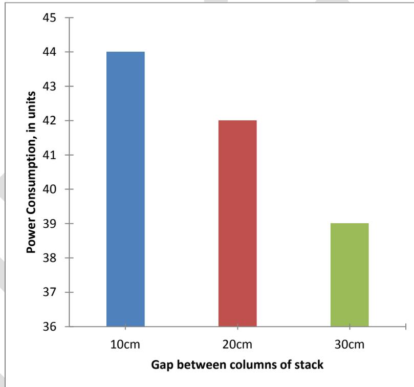
**Figure 18** Power consumption of cold storage in three different stacking arrangements
