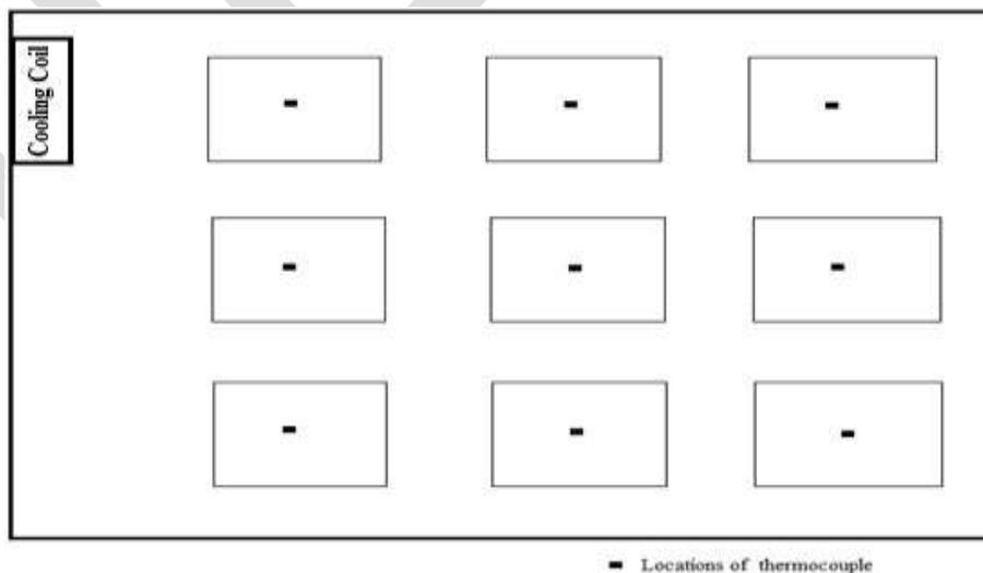
*Figure 7* Different Locations of T-type Thermocouple on a Plane from Top View
