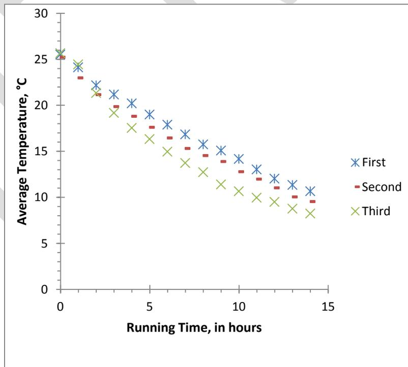
**Figure 17** Overall Average Temperature Distributions in Cold Storage for Different Arrangements
