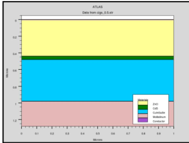
**FIG. 1.** DEVICE STRUCTURE USED FOR SOLAR CELL SIMULATION USING SILVACO ATLAS SIMULATION SOFTWARE.
