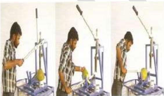
**Fig 3 : Manual operated punch cum splitting the tender coconut machine**
