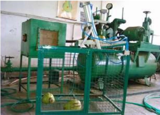
Fig 5 : Working model of punch cum splitter for tender coconut
