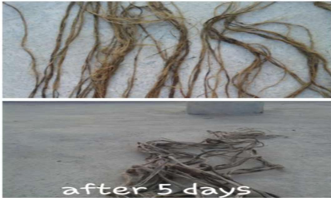
**Fig.2 Treated fibre is dried in sunlight for 48 hrs**
