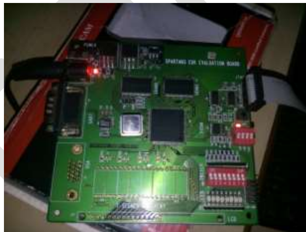
Figure 7: Xilinx Spartan 3 FPGA kit
