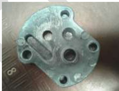
Figure No: 4.3 Flange Lube Oil Pump Filter
