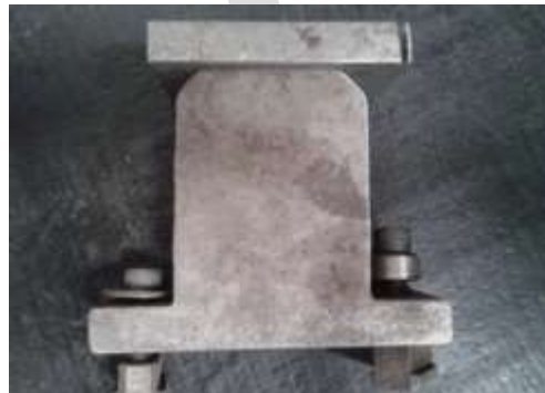
Figure No: 4.2 Front View of previous fixture
