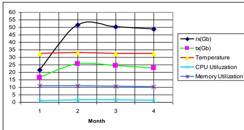
Figure 6. Performance of Router 2 after 6 months with 256Mb RAM open chassis and with proper cooling
