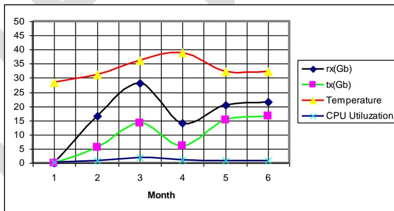
Figure 5. Performance of router 2 for with 128MB RAM, closed chassis
