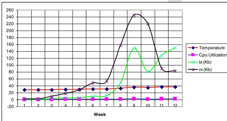
Figure 4. Performance of router 1 with 256MB RAM, closed chassis
