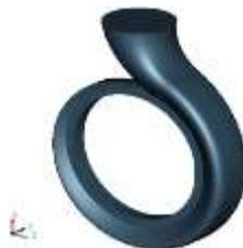
Fig.3: 3D model of a centrifugal pump volute fluid volume.
