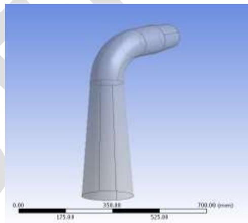
Fig.5: Draft tube fluid volume.
