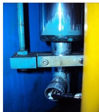
Fig. 7. The stroke transducer
