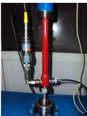
Fig. 5. The pressure and temperature transducer.
