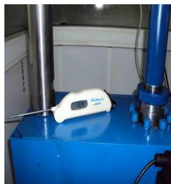
Fig. 8. The ambient thermometer
