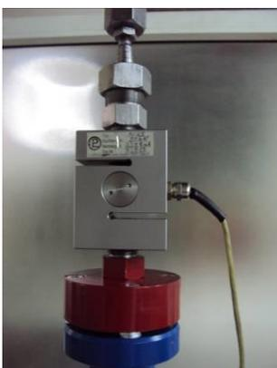
Fig. 6. The force transducer.
