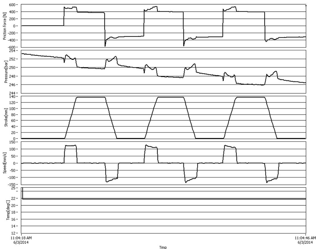
Fig. 13. The complex characteristic graphs for pressure step values of 250 bar.
