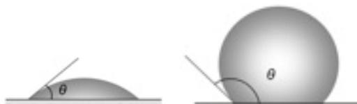
**Figure 2: Super-Hydrophilic (Left) and Super-Hydrophobic (Right) Surfaces**
