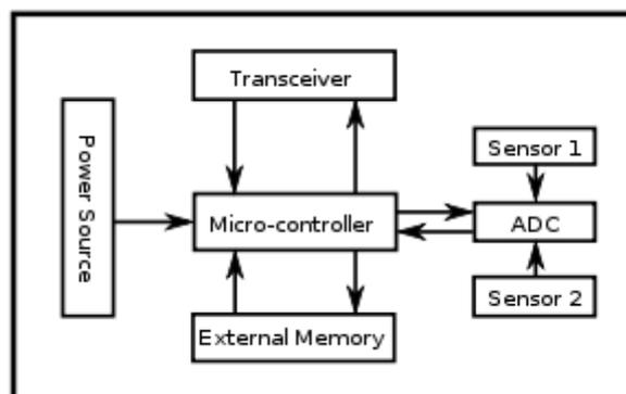
Fig. 2 components of sensor node
