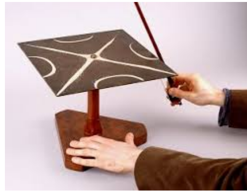
Fig. 4. Formation of standing waves by the excitation of a metal plate by a bow. Note that, the salt crystals are pushed to the stationary nodes [16].
