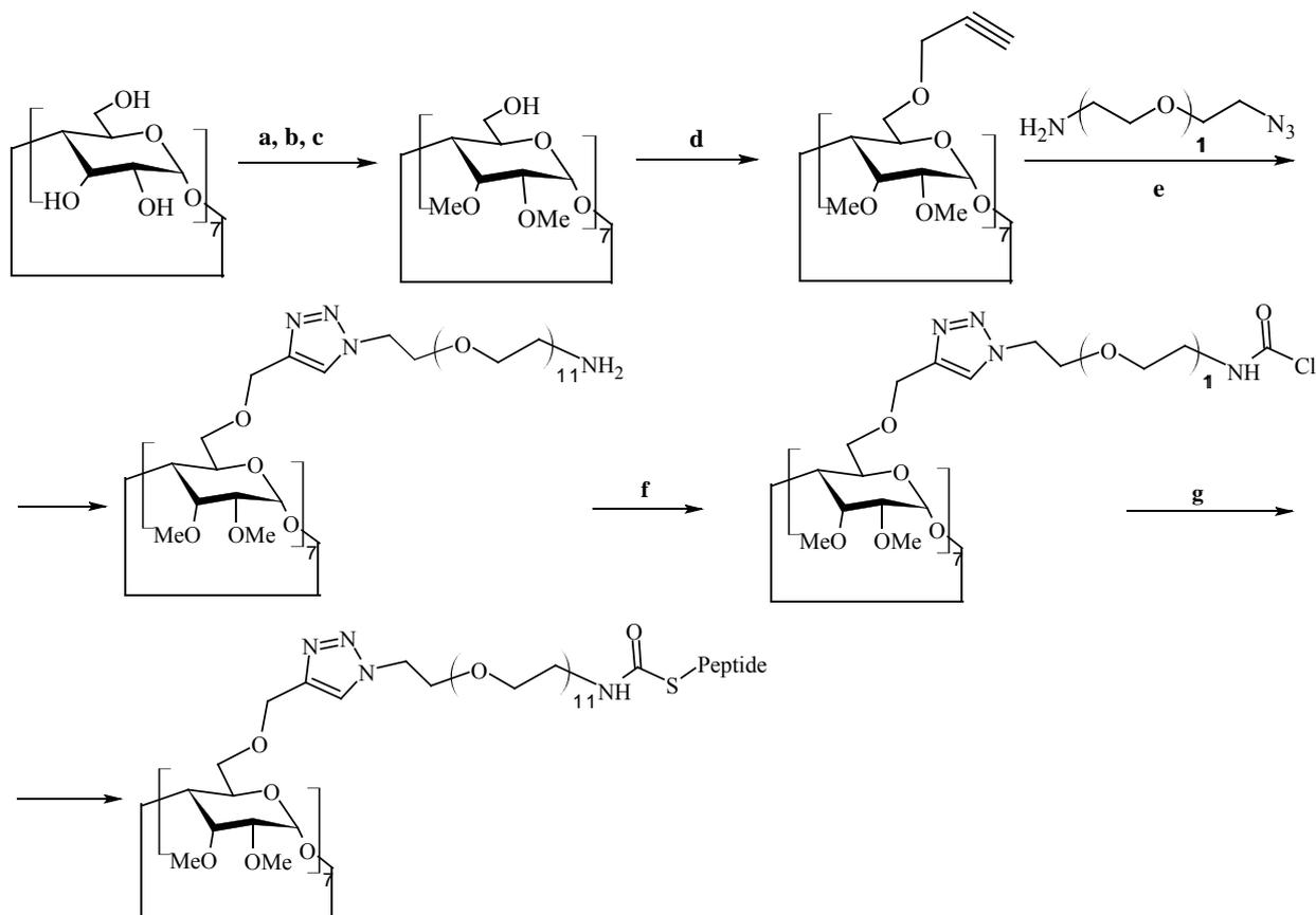
**Fig. 6.** Scheme of synthesis of heptavalent anthrax toxin inhibitor. (a) TBDMSCl, pyridine, 0°C - rt.; (b) NaH, MeI, THF; (c)  $\text{NH}_4\text{F}$ , MeOH, reflux; (d) NaH, propargyl bromide, DMF, 0°C - rt. (e)  $\text{CuSO}_4$ , sodium ascorbate, THF:H<sub>2</sub>O:BuOH (0.5:1:1), 80°C; (f) chloroacetic anhydride, triethylamine; (g) peptide, DMF, DBU, triethylamine [22].
