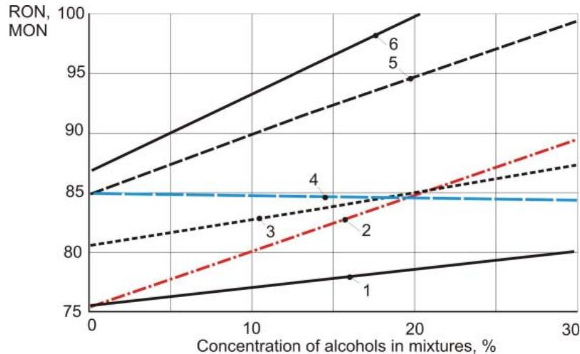
Fig. 2. The dependence of the octane number of biofuel mixtures on the alcohol concentrations: 1, 2, 3, 4 -  $COM = f(C)$ , 5, 6 -  $COR = f(C)$ , 1 - butanol + gasoline A-80, 2 - ethanol + gasoline A-76, 3 - ethanol + gasoline A-80, 4 - E16B16 mixture, 5 - ethanol + gasoline A-80, 6 - ethanol + gasoline A-90
