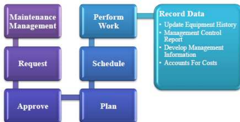
Figure 2. Maintenance management flowchart
