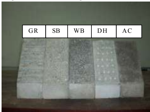
Fig. 2: Slant shear test specimens with the different surface textures
