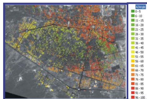
Fig. 5: Parcel azimuth angle for the most visible walls (radar specific)
