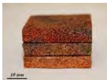
Fig. 1: Copper foams with the same \epsilon and different d_{\text{cell}} (40, 50 and 65 ppi respectively from top to bottom)
