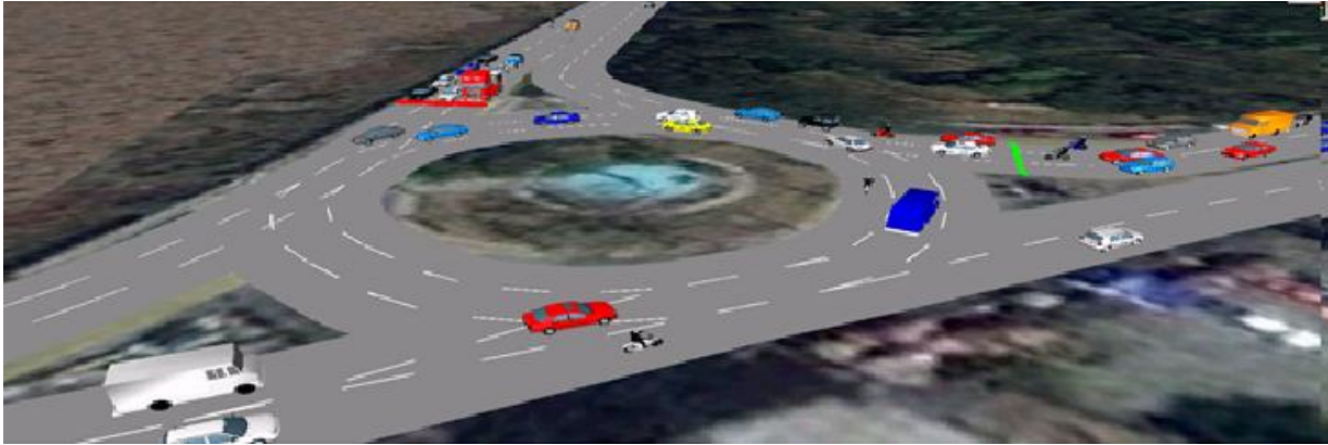
Figure 2. A screenshot of an example microsimulation run on BR using VisSim as a simulation visualization framework. The red line across the road means that the vehicles coming from that direction are stopped, while the green line means that the vehicles are moving.
