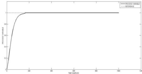
Figure 10- FMPC response (tank 1)
