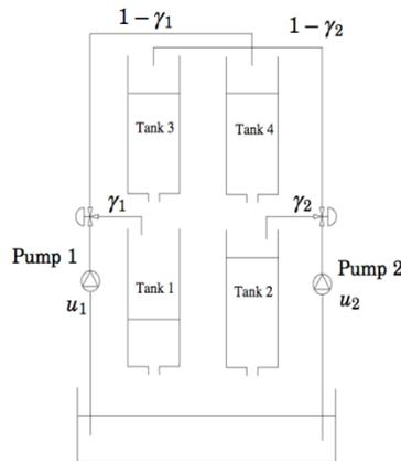
Figure 1 Setup of quadruple tank system
