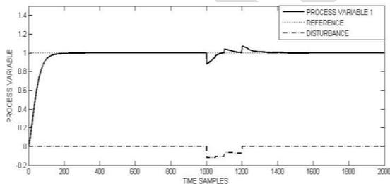
Figure 6- Disturbance rejection
