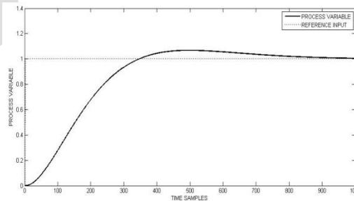
Figure 2- PID response – SISO
