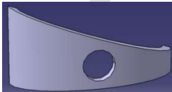
Fig: 1.2 Curved Trapezoidal Winglet with hole (CTWH)
