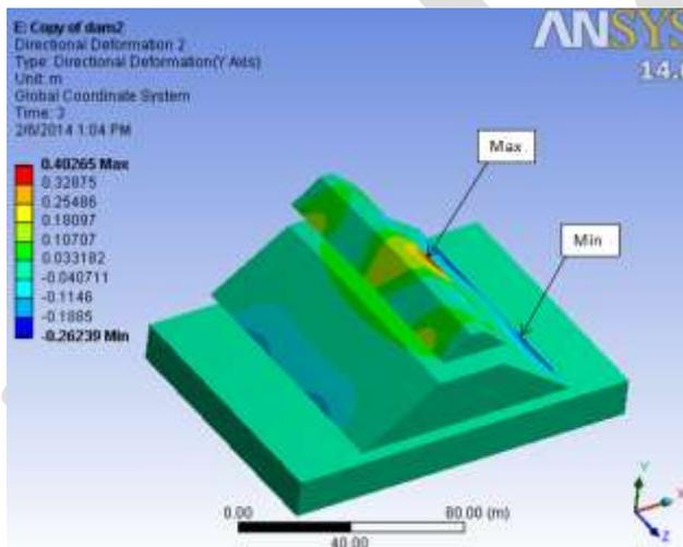
Figure 8. Minimum and maximum of dynamic vertical displacement of Dam 1
