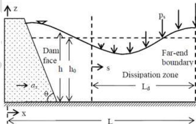
Figure 1. Definition sketch of dam-reservoir system subjected to earthquake
