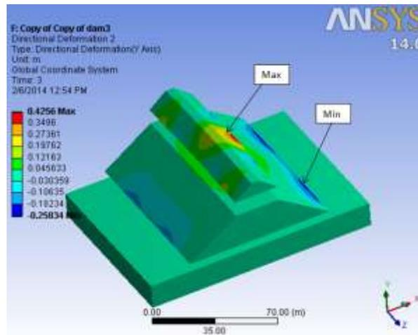
Figure 10. Minimum and maximum of dynamic vertical displacement of Dam 3
