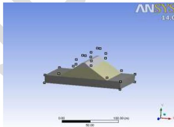
Figure 2. geometry of dam and foundation
