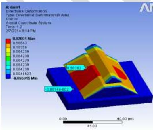
Figure 5 . Minimum and maximum of dynamic horizontal displacement of Dam 1
