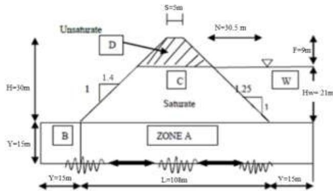
Figure 3.the geometrical dimensions ofDam
