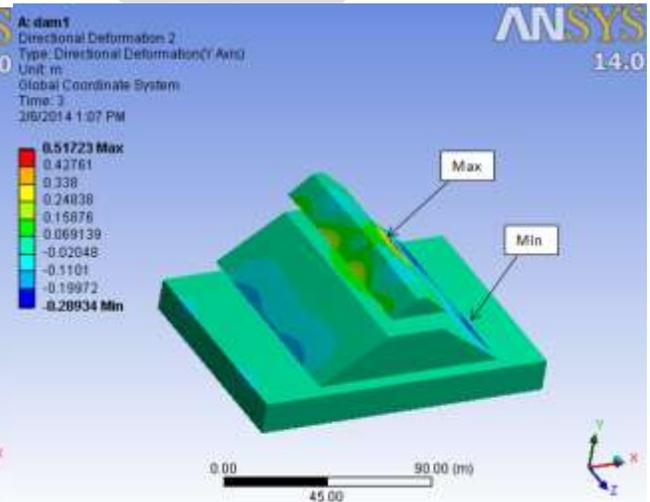
Figure 9. Minimum and maximum of dynamic vertical displacement of Dam 2
