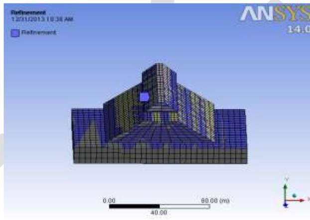
Figure 4.used Mesh for model
