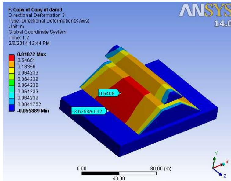
Figure 7. Minimum and maximum of dynamic horizontal displacement of Dam 3
