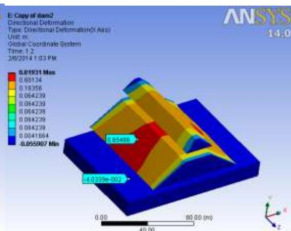
Figure 6. Minimum and maximum of dynamic horizontal displacement of Dam 2
