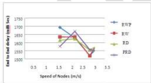
Fig 4 End-to-End Delay vs. Speed of Nodes
