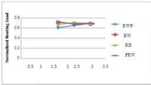
Fig 3 normalized Routing Load vs. Speed of Nodes
