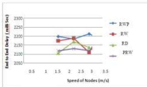
Fig 9 End-to-End Delay vs. Speed of Nodes
