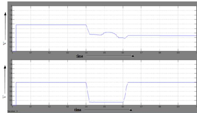
**Fig. 18.** Voltage  $V_{RMS}$  at load point after the occurrence of three phase fault without D-STATCOM.
