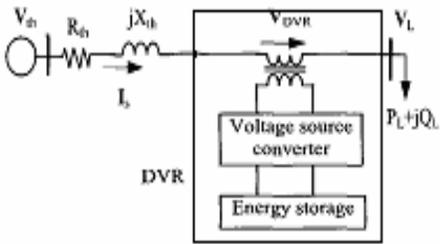
Fig. 1. Schematic diagram of a DVR.
