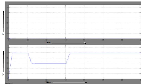
**Fig. 10.** Voltage  $V_{RMS}$  at load point after the occurrence of Double Line to ground fault without DVR.
