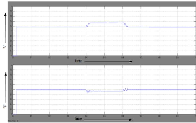
**Fig. 17.** Voltage  $V_{RMS}$  at load point after the occurrence of Double Line to ground fault with D-STATCOM Energy storage of 35 KV.
