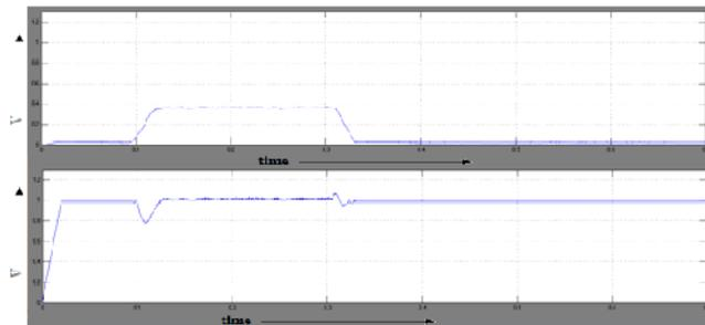
**Fig. 13.** Voltage  $V_{RMS}$  at load point after the occurrence of three phase fault with DVR Energy storage of 7 KV.
