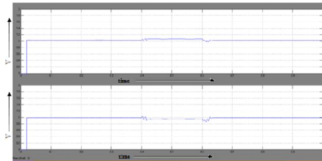
**Fig. 15.** Voltage  $V_{RMS}$  at load point after the occurrence of Single Line to ground fault with D-STATCOM, Energy storage of 25 KV.
