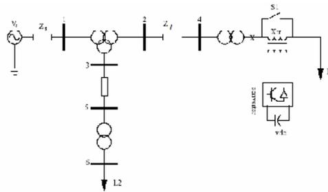
Fig. 2. Single line diagram of the test system for DVR.
