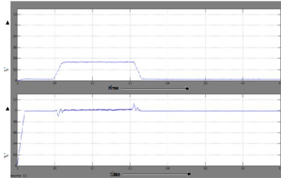
**Fig. 11.** Voltage  $V_{RMS}$  at load point after the occurrence of Double Line to ground fault with DVR Energy storage of 7 KV.
