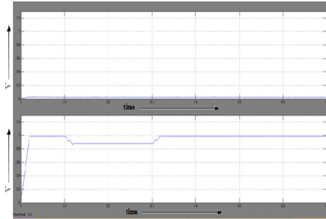
**Fig. 8.** Voltage  $V_{RMS}$  at load point after the occurrence of Single line to ground fault without DVR.
