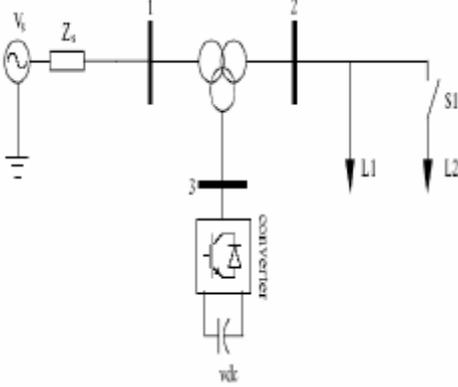
**Fig. 5.** Single line diagram of the test system for D-STATCOM.
