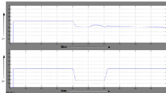
**Fig. 16.** Voltage  $V_{RMS}$  at load point after the occurrence of Double Line to ground fault without D-STATCOM.
