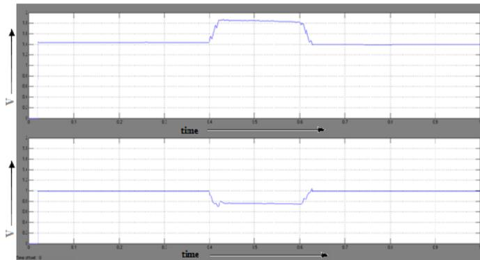
**Fig. 19.** Voltage  $V_{RMS}$  at load point after the occurrence of three phase fault with D-STATCOM Energy storage of 35 KV.
