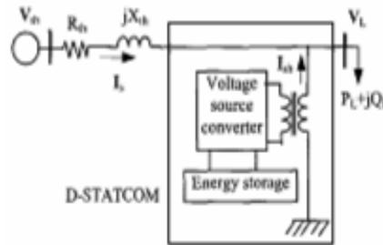
Fig. 4. Single line diagram of the test system for D-STATCOM.
