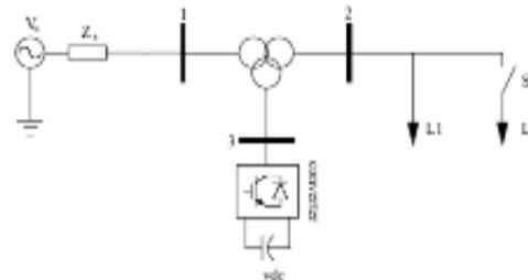
**Fig. 6.** Single line diagram of the test system for D-STATCOM.
