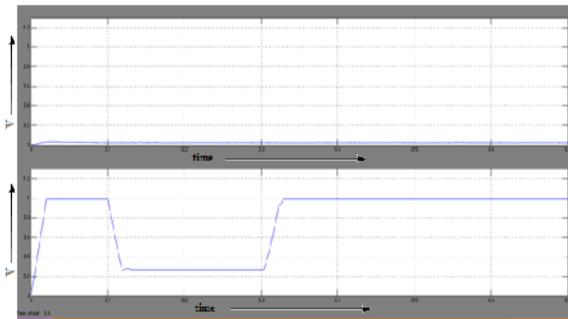
**Fig. 12.** Voltage  $V_{RMS}$  at load point after the occurrence of three phase fault without DVR.
