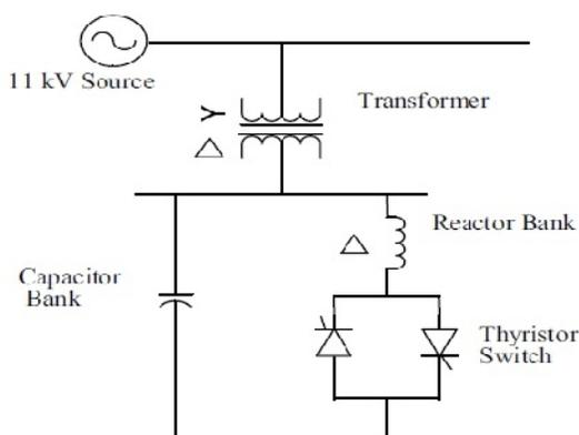
Fig. 1. The SVC diagram of exchange power from the ac system.
