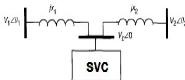
Fig. 3. Three bus system model with SVC.
