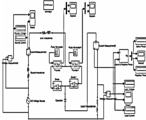
**Fig. 13.** SSSC Compensated System.
