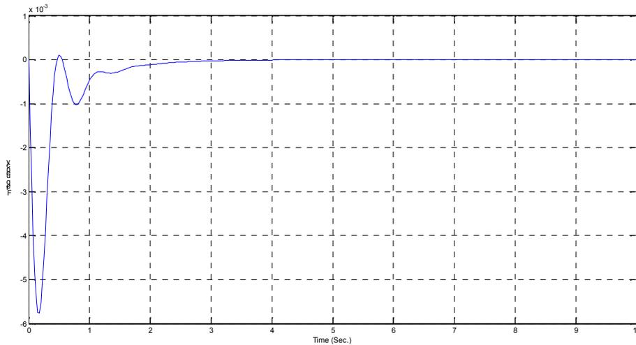
**Fig. 6.** Deviation of frequency of the single area power system with PSO based PID controller.
