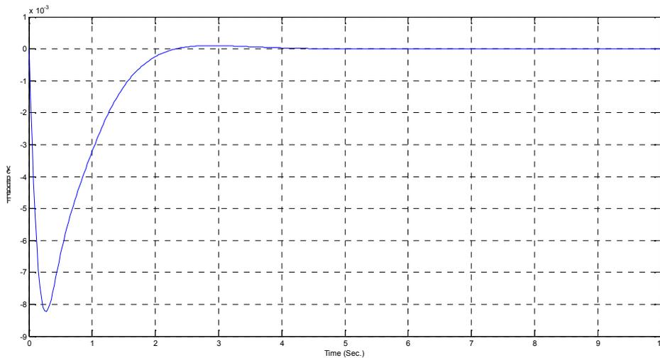
Fig. 5. Deviation of frequency of single area power system with GA based PID controller.
