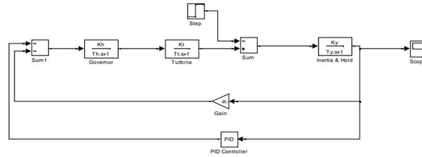
Fig. 4. Single area power system with proposed PSO and GA based PID controller.
