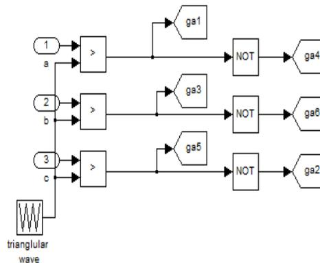
Fig.5. Triangular carrier block to obtain PWM signals for VSI.
