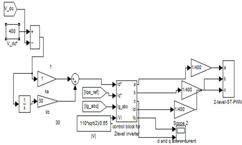
Fig. 4. Matlab transformation block (dq0-abc) for PWM signal generators of VSI.
