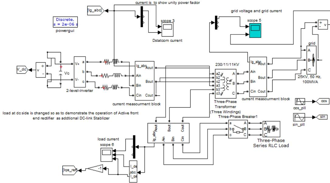
Fig. 3. Matlab model of the DSTATCOM.
