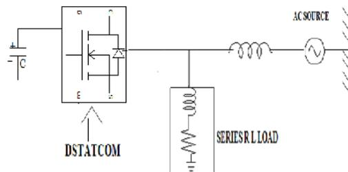
**Fig. 1.** Basic components of DSTATCOM circuit.
