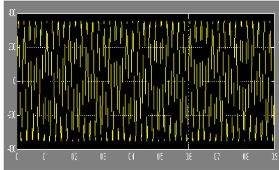
Fig. 10. Output waveform of the load voltage with DSTATCOM.
