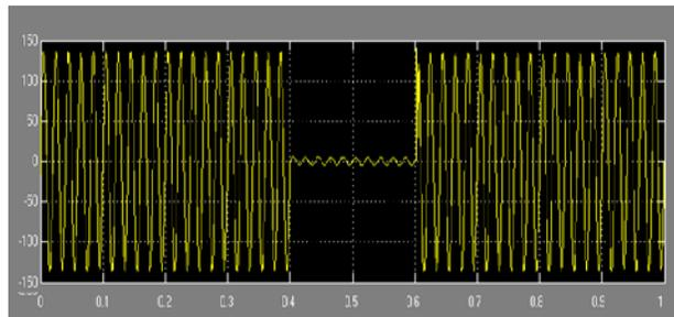
**Fig. 9.** Output waveform without DSTATCOM showing the result of short circuit.
