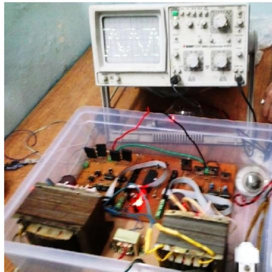
Fig.7. Complete hardware set-up cascaded H-bridge 5-level PWM inverter for single phase IM.
