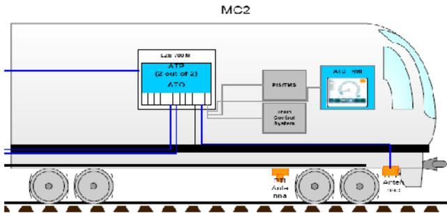
**Fig. 7.** Onboard signalling equipment.
