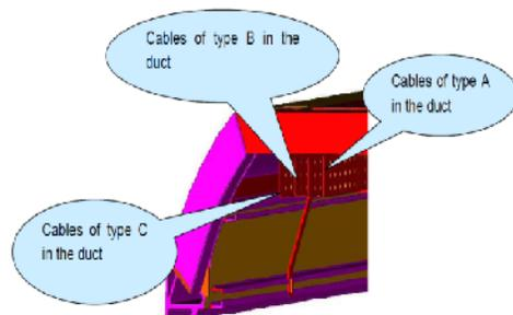
Fig. 6. Different type of cables are placed in ducts with partitions.
