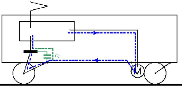
**Fig. 10.** Technique to reduce harmonics using capacitor.
