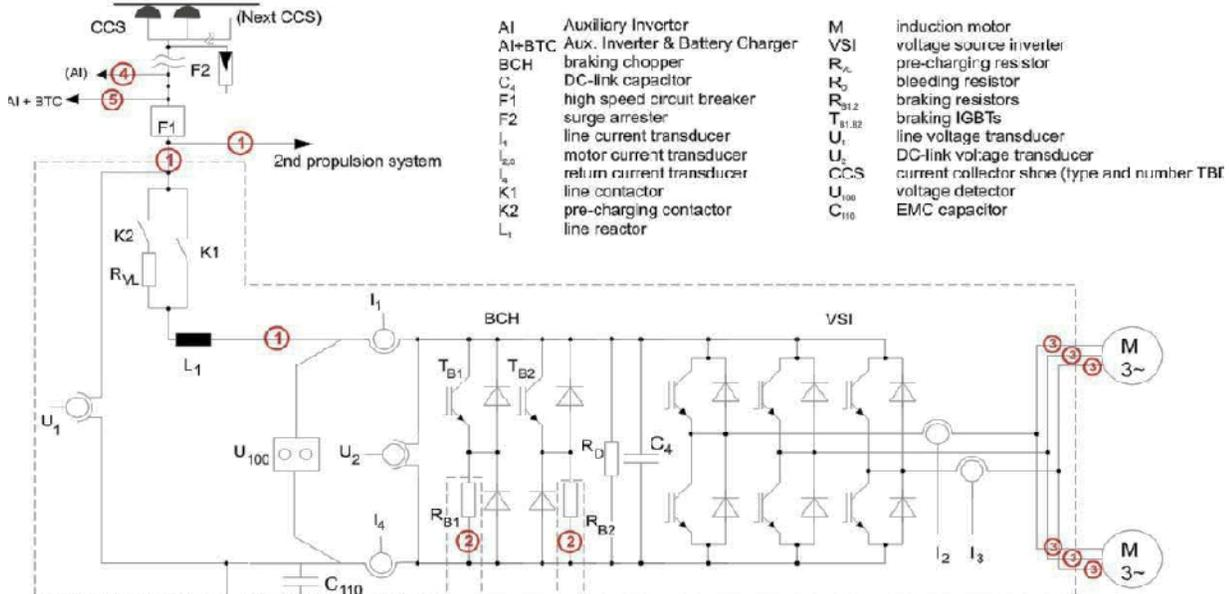
Fig. 5. Schematic diagram of DC traction system.
