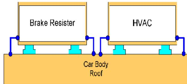
Fig. 4. Equipment bodies earthed in a rolling stock.
