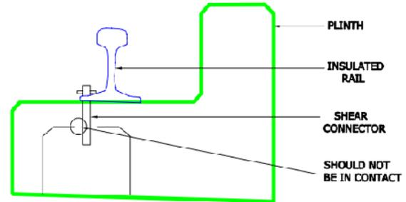
**Fig. 11.** False "occupied" status for track circuits.
