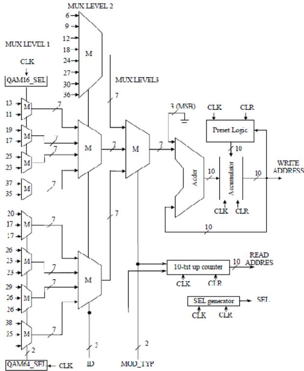
Fig. 1. WiMAX Address generator.
