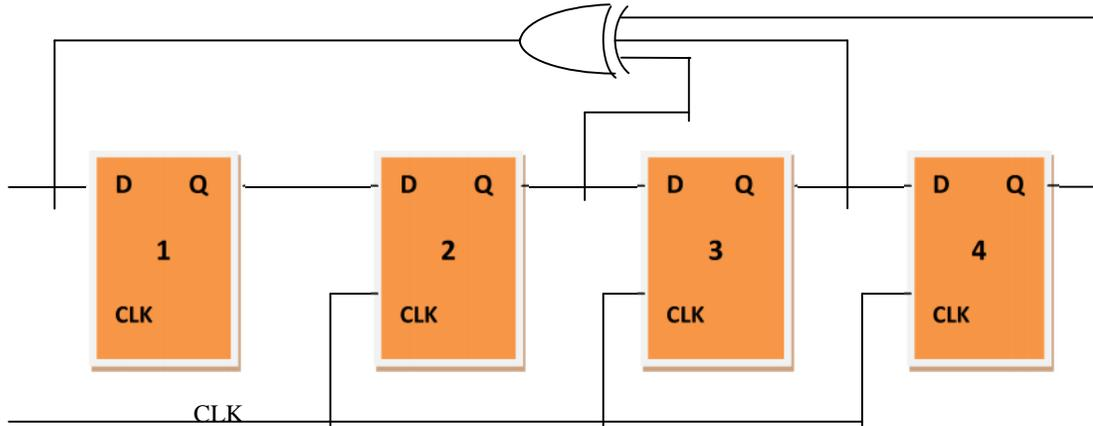
Fig. 3. Logic Diagram of Pseudo Random Binary Sequence Generator.
