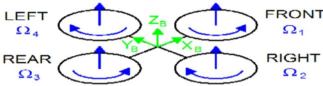
Fig. 1. Quad-rotor motor in hovering.
