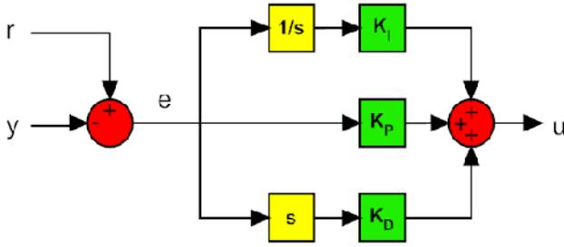
Fig. 2. Traditional PID structure.
