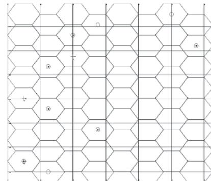
Fig. 4. Channels Allocated in Hexagonal Structure .Four Channels are taken in the figure to demonstrate the frequency reuse concept as one channel appear once only in a cluster.
