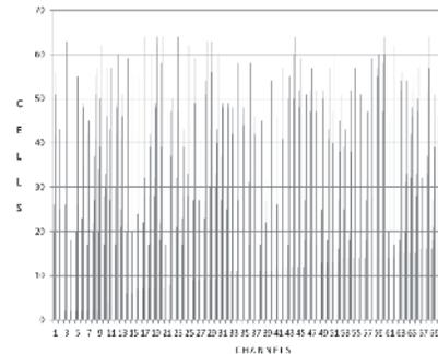
Fig. 3. Channels Allocated to cells. Each channel is allocated in five to six cells that are far apart satisfying the constraints.
