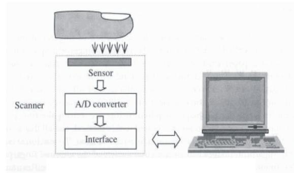
Fig. 9. General structure of scanner.
