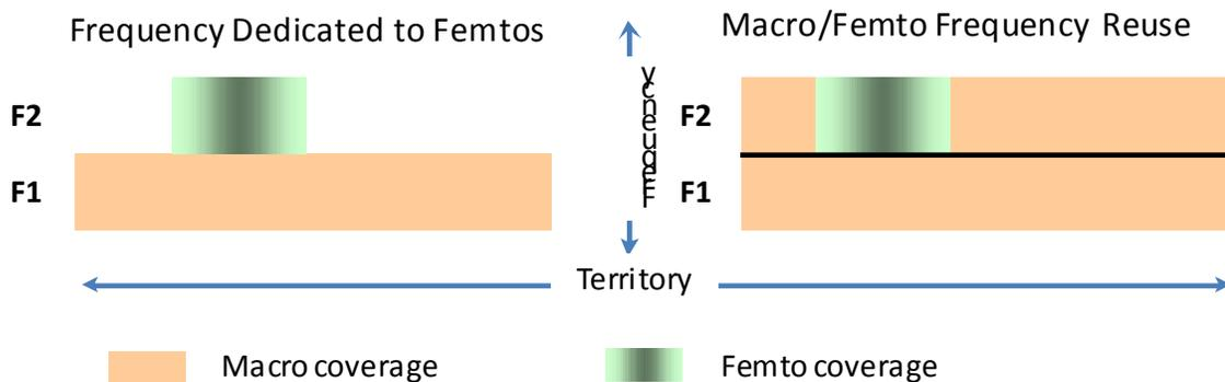
Fig. 3. RF deployment scenarios for femtocell systems.
