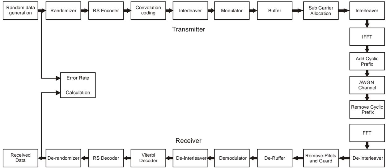
Fig. 1. Physical Layer Block Diagram based on IEEE802.22 WRAN.
