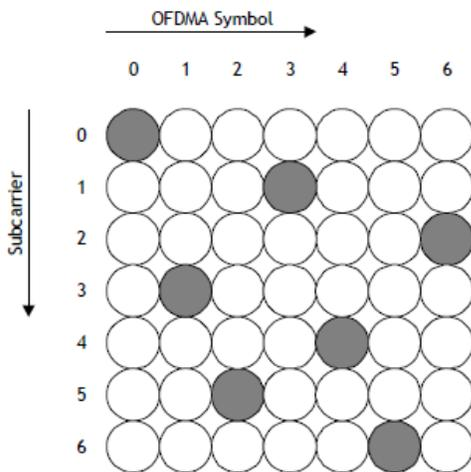
Fig. 2. Pilot insertion pattern.
