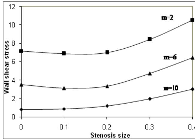
**Figure 5: Variation of Wall Shear Stress with Stenosis Size for different Values of m**
