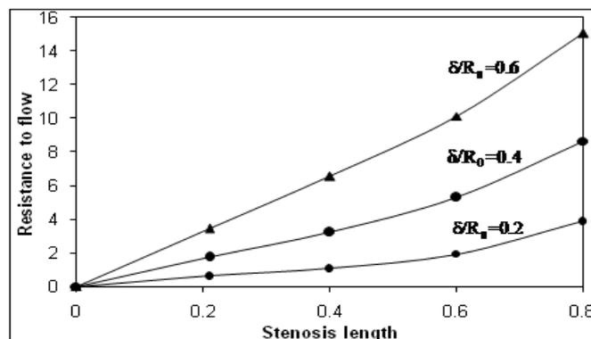
Figure 4: Variation of Resistance to Flow with Stenosis Length
