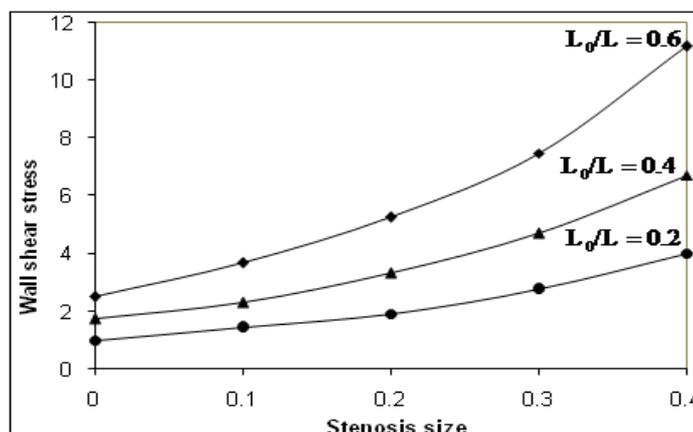
**Figure 6: Variation of Wall Shear Stress with Stenosis Size for Different Values of Stenosis Length**
