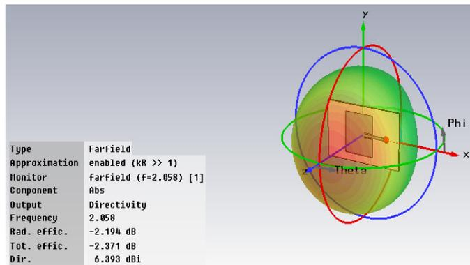
Figure 3: Radiation Pattern of RMPA Showing 76.29% Total Efficiency & 6.393 dBi Directivity
