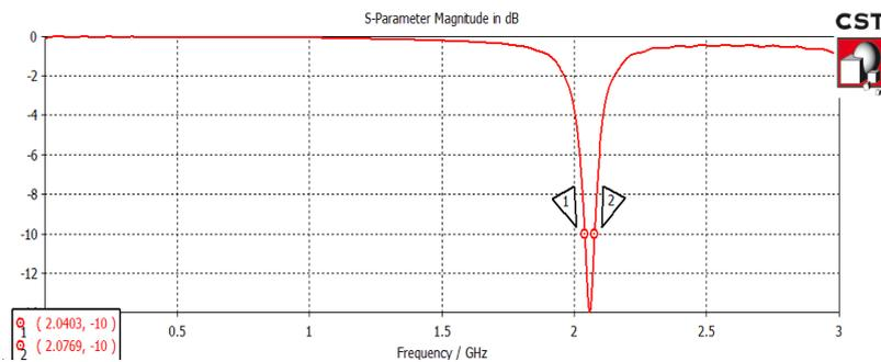
Figure 2: Simulated Result of RMPA Showing Return Loss of -14 dB and BW of 36.6 MHz
