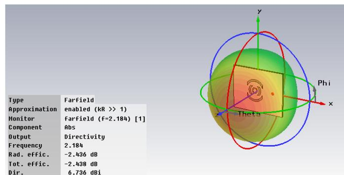
Figure 6: Radiation Pattern of the RMPA along with the Suggested Material Cover Showing Total Efficiency of 75.62% and the Directivity 6.736dBi
