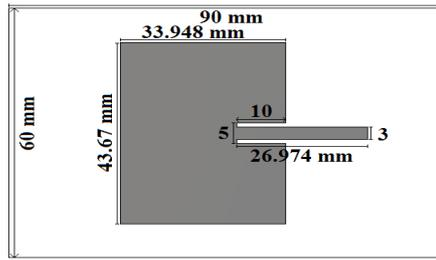
Figure 1: Dimensional View of RMPA at 2.058 GHz (All Dimensions in mm)
