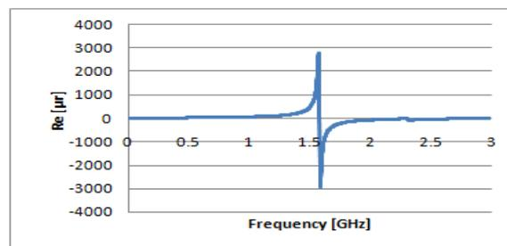
Figure 9: Permeability versus Frequency Graph
