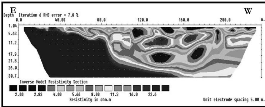
**Figure 5:** Tomography of resistivity of the second profile
