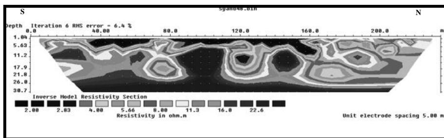
**Figure 4:** Tomography of resistivity of the first profile
