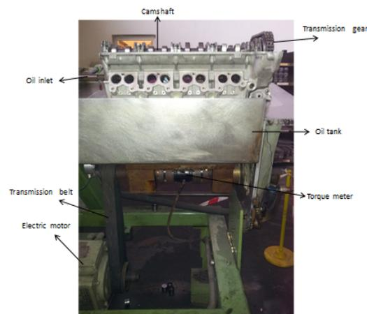
Figure 3. Camshaft wear test machine
