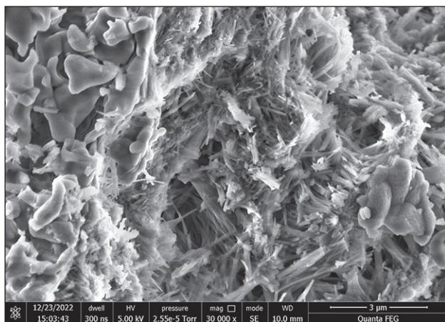
Fig. 5. Formation of a needle-like structure of the multifunctional additive “Betomix-ITH Gel”, magnification  $\times 30000$
