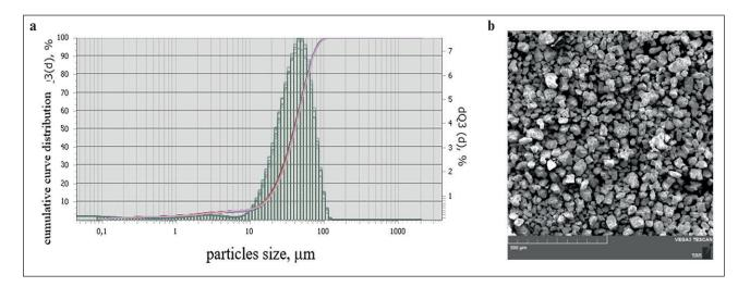
Fig. 2. a) particle size distribution of the additive; b) microphotograph of the additive particles
