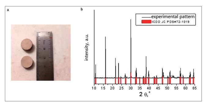
Fig. 1. a) additive pressed into pellets b) XRD pattern of the additive
