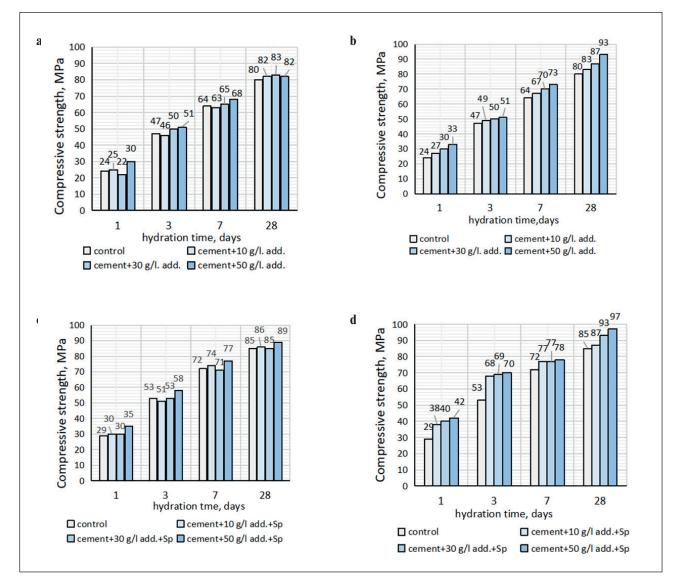
Fig. 3. **Compressive strength of the samples depending on the hydration time:** a) I – by dry mixing of cement and the additive, followed by mixing with tap water; b) II – by mixing cement powder with water suspensions of the additive after ultrasonication; c) III – by dry mixing of cement and additive, followed by mixing with water-plasticizer solution; d) IV – by mixing the cement powder with water-polymer suspension of the additive stabilized by ultrasonic processing
