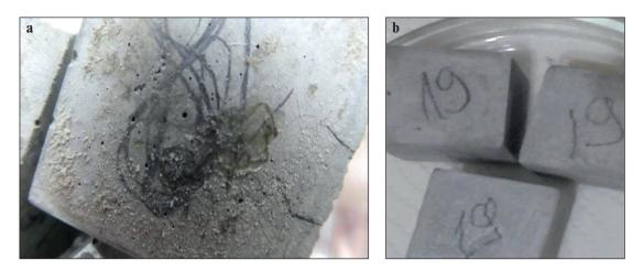
Fig. 5. Control (a) and modified (b) cement stone samples after being kept in suspension of fungi spores for 3 months
